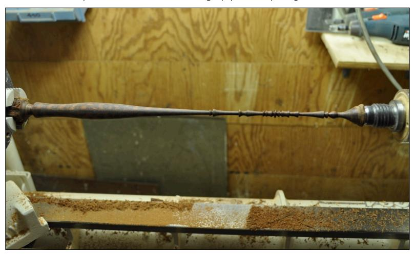
Excess wood is cut off at the tail stock to allow the finishing of the finial.
