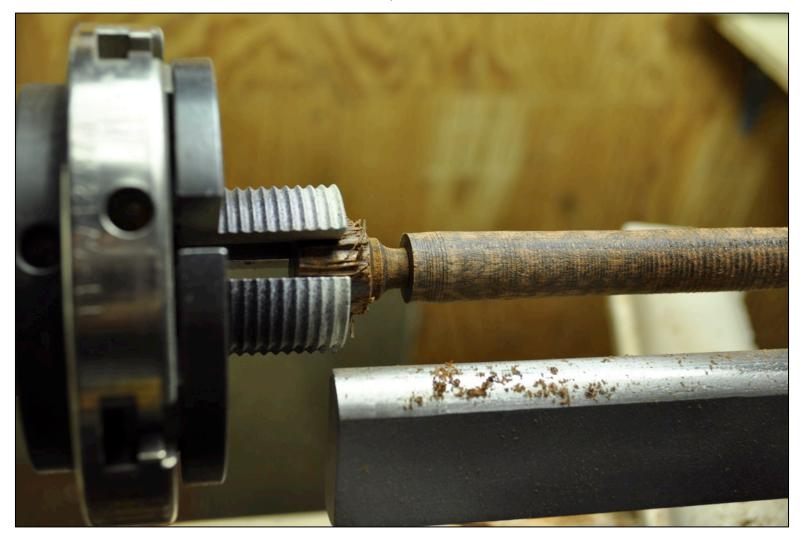
Spinning at 1500 RPM some contours of the pen are being created.
