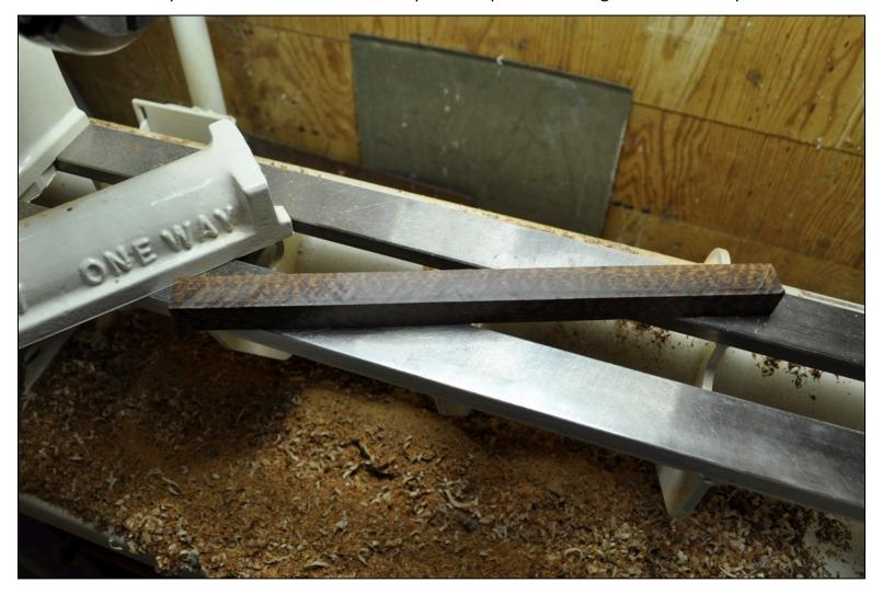
Set into a four jaw chuck and live end tail stock for balanced, smooth turning.
