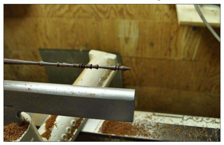
Once cut from the lathe a slot is cut into the pen in order to receive a brass flange.
