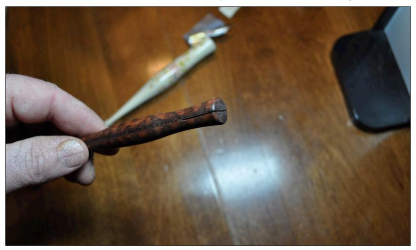
The flange is glued into place with a dummy nib inserted to aid in the coating process.
